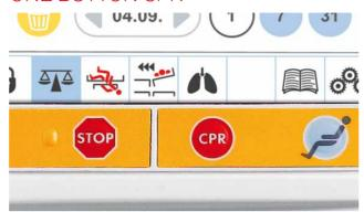
One touch CPR simultaneously flattens the bed frame and deflates the air mattress. There is also a manual CPR release on the mattress for quick deflate during transport.
